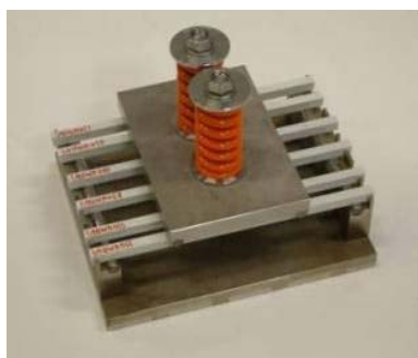
Figure 9: Self-stressing four-point flexure test fixture with GRP specimens.
